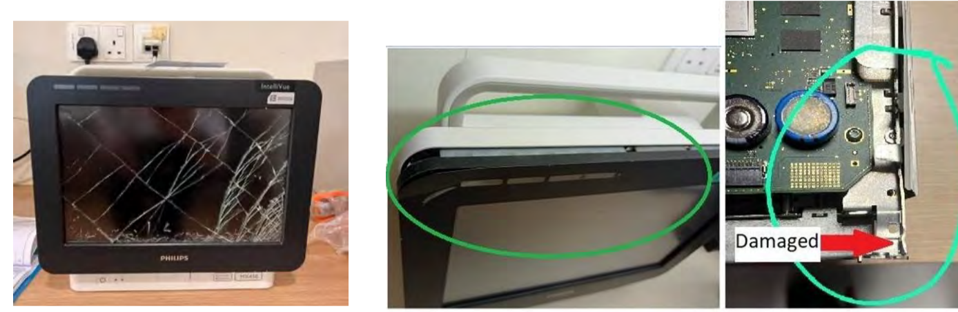
Broken touch screen Repair cost: $347.00 Damaged touch screen and internal enclosure Repair cost: $1,075.73
